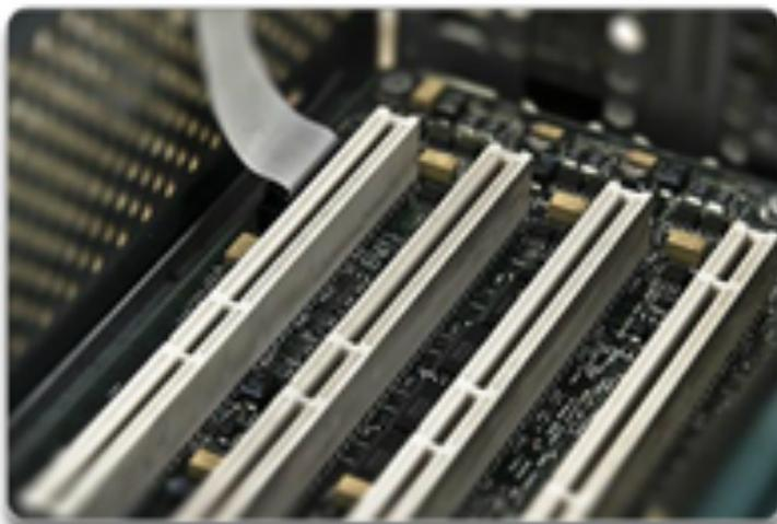
PCI-Extended is a 32-bit bus with higher bandwidth than the PCI bus. PCI-X can run up to four times faster than PCI.
