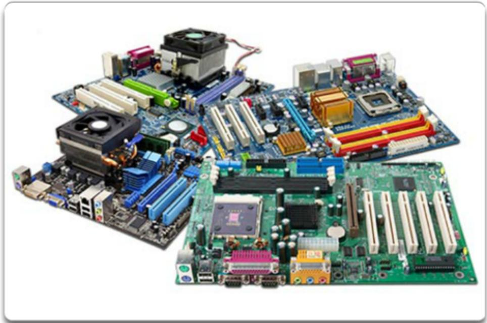
The motherboard accommodates the central processing unit (CPU), random access memory (RAM), expansion slots, heat sink and fan assembly, basic input/output system (BIOS) chip, chipset, and the circuitry that interconnects the motherboard components. Sockets, internal and external connectors, and various ports are also placed on the motherboard.
