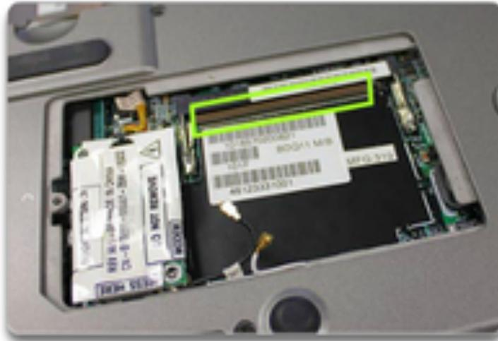
Mini PCI is a 32-bit bus used by laptops. Mini PCI has three different form factors, Type I, Type II, and Type III.
