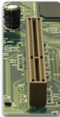
AGP is designed to be used by video adapters. Advancements in the specification for AGP allow for bandwidth increases. The bandwidth of the port can be multiplied 2X, 4X, or 8X.
