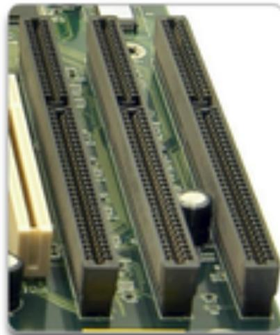
Industry Standard Architecture is an 8-bit or 16-bit expansion slot. This is older technology and is seldom used.
